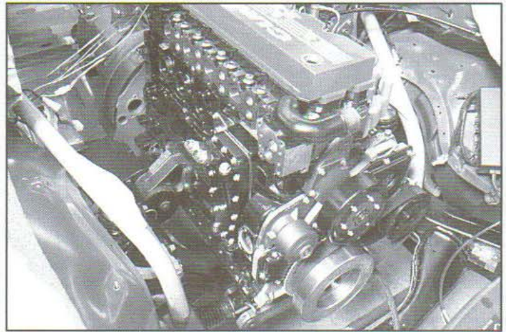
The engine of choice for the project was the "anvil strong" Cummins ISB 24-valve 5.9L engine. Diesel engines have long-held negative performance connotations in many racing circles. Maybe it would help to call them compression ignition engines instead.
