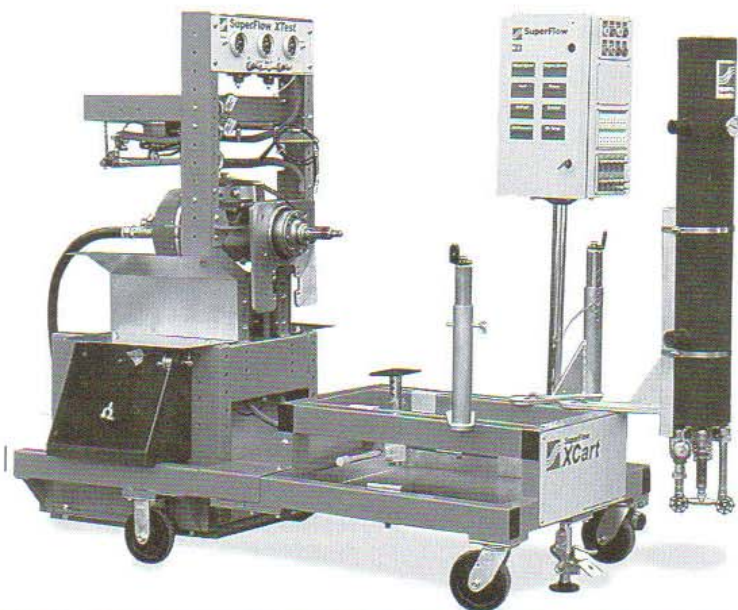
An engine dynamometer provides a direct measurement of developed engine torque (and therefore horsepower) with no external influence from other vehicle aspects, such as driveline losses. Engine dynos are most often used for research, endurance testing, reliability measurements, and determining exact engine outputs for engineering and marketing purposes. (SuperFlow)
