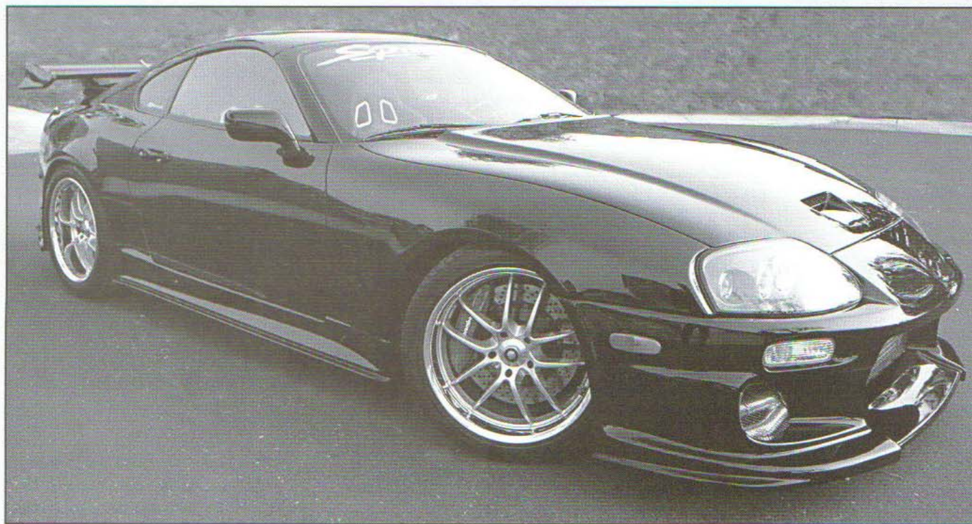
The car has been fitted with a body kit with a larger-than-stock intercooler opening and a hood scoop that allows ambient air directly into the engine compartment. The engine generates over 1000 hp at the drive wheels, but the vehicle can operate effortlessly with power windows and the air conditioning without fear of overheating in California's dreaded bumper-to-bumper traffic.
