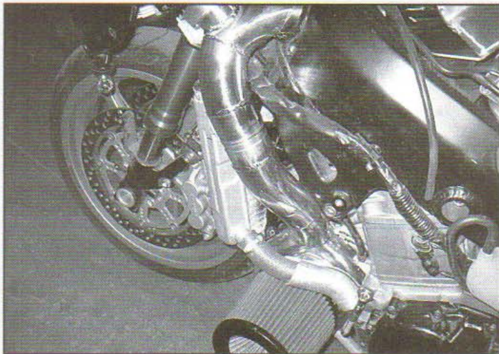
The compressor-side of the turbocharger system. The blow-off valve is mounted at the top of the up-pipe.
