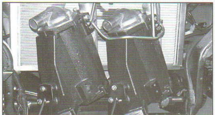
Dual Cummins marine air-to-water charge air coolers, plumbed in parallel. Excellent performance was obtained with efficiencies in the 90% range with less than 0.5 psi total pressure drop. Air temperatures went from over 500 degrees Fahrenheit at the compressor outlet, to approximately 100 degrees F in the intake manifold. These intercoolers cost $5,000 apiece.
