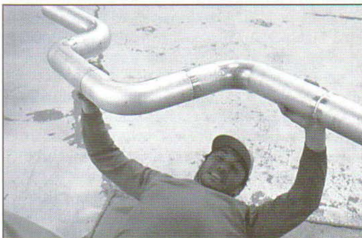
The exhaust system is fabricated from 4-inch aluminum 6061 tubing. Total weight is just 10.5 pounds. It's not as heavy as this guy makes it look.
