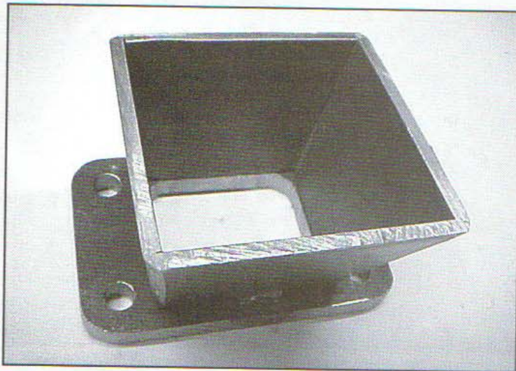
The collector is trial-fitted together with tack-welds.
