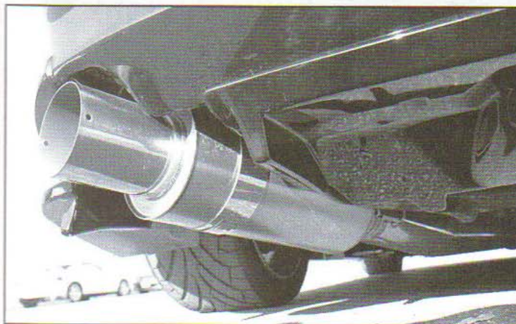
While certainly pretty, the titanium HKS exhaust system on this Supra was chosen solely for its flow characteristics and low backpressure. (Henderson / SP Engineering)
