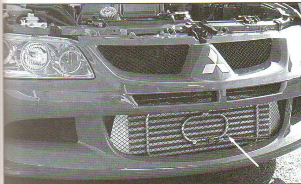
CO 2 spray bars like this can help lower the intercooler core temperature. Just make sure the CO 2 doesn't end up being ingested by the engine intake system. (Design Engineering, Inc.)
