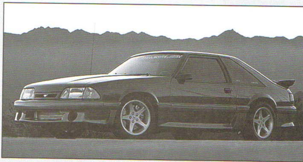
This unassuming Fox-bodied Mustang GT serves double duty as a weekday daily driver and weekend racer. A single-turbo system delivers 700 hp and 700 lb-ft of torque to the rear wheels. The only exterior hint of the turbo system is the intercooler nestled into the front bumper.
