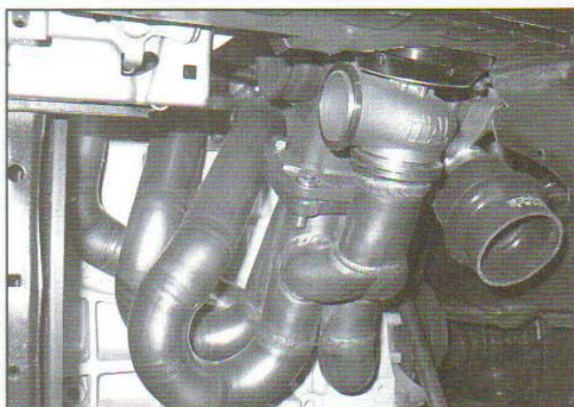
A key part of generating reliable mega-horsepower is a well-engineered exhaust manifold. Individual runners were sized to deliver equal and maximum pressure pulses to the turbine. Wastegate is a TIAL 44 mm unit.
