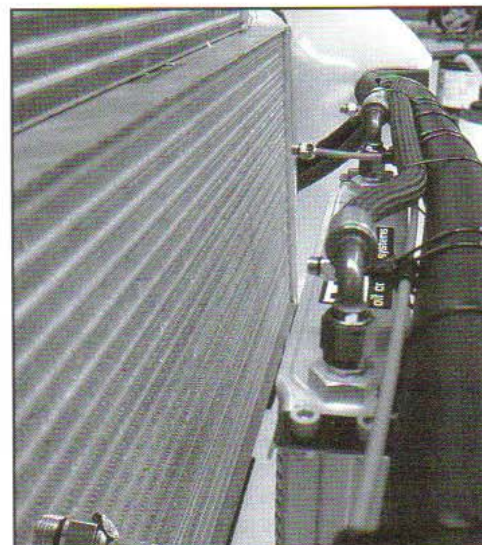
A water spray device can increase the effectiveness of an intercooler. In exactly the same way that evaporating sweat removes heat from the skin of a human body, water that is sprayed onto the surface an intercooler will vaporize and remove heat energy. Note, however, that many race venues won't let cars with water spray devices onto their tracks, because the devices are technically considered a fluid leak. There is also the added weight of the water, tank, pump, and supply lines to consider. (Aquamist)
