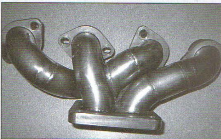
The stainless steel exhaust manifold during construction. Tube diameters are 1.5-inches.
