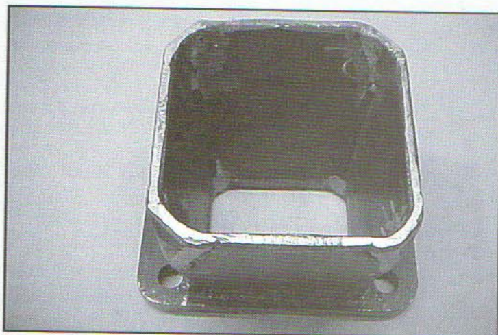
The entrance corners of the collector are then reworked to mate with the round runner tubes. This step helps ensure a less-turbulent gas flow transition from the runners to the collector.
