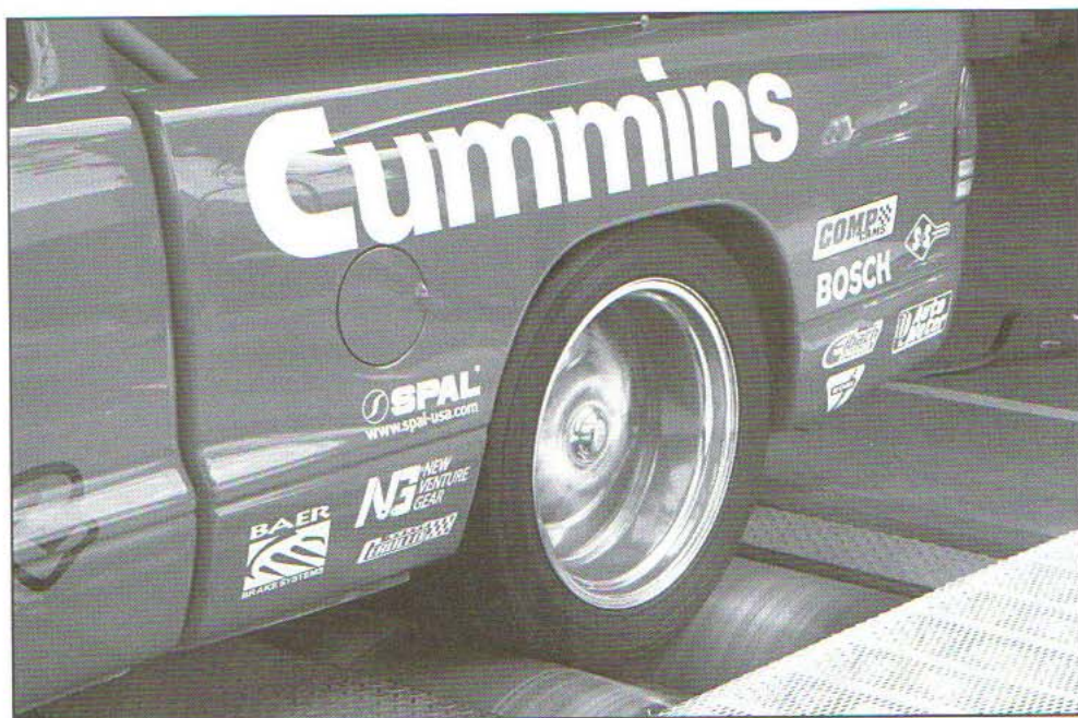
The same turbo-diesel being tested in its vehicle on a chassis dynamometer. The luxury of testing both on an engine and chassis dyno can allow engineers to quantify driveline losses and help optimize the overall vehicle setup for a specific race application. (Gale Banks)
