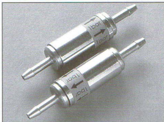
Check valves are used to keep water flowing in only one direction under boost. Good filtration is necessary, however, as small foreign objects can cause these devices to malfunction. (Aquamist)
