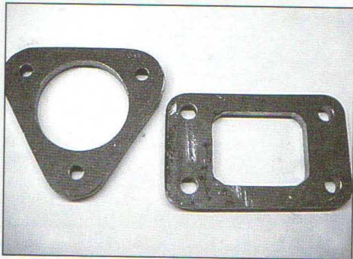
A mounting flange for the turbine is cut from 1/2-inch flat stock.
