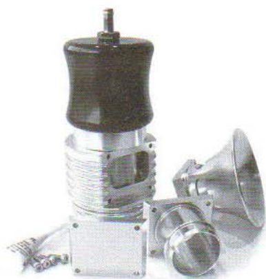
A configurable blow-off valve. This unit can be changed from BOV to BPV by simply switching the outlet port fitting. (Turbosmart)
