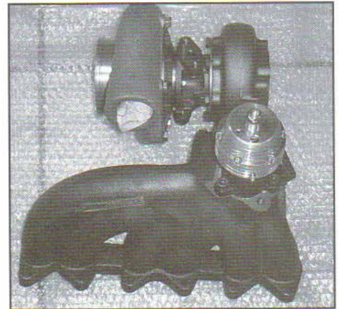
A compact log manifold for a six-cylinder engine. (The Power Group)
