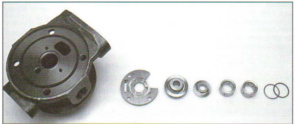
A conventional journal bearing stack up. Note the 360-degree thrust bearing. (Turbonetics)
