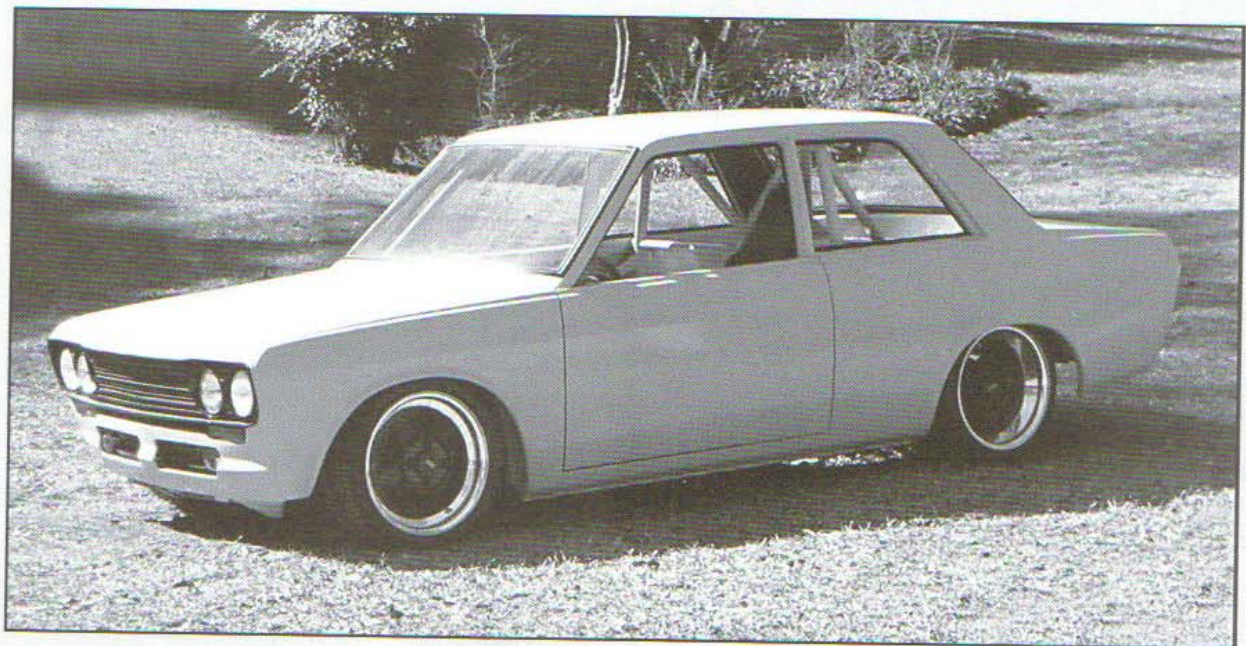
1969 Datsun 510 with turbocharged Mazda rotary engine. Horsepower was added and vehicle mass reduced, improving both numerator and denominator in the quest for a maximum power-to-weight ratio.
