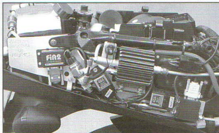
Where space is tight, clever packaging is required. This Suzuki Hayabusa has a complete water injection system mounted underneath the seat and rear valance. (Aquamist)
