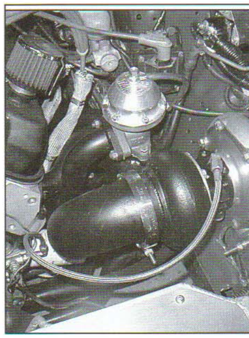
Whether journal or ball bearing-equipped, all CHRAs require a steady supply of clean, filtered oil. Many aftermarket turbo systems tap into the oil pressure sending port on the side of the engine block. A simple "T" arrangement ensures sufficient oil to the turbocharger. Note the use of a high-quality braided stainless steel hose on this single-turbo Ford Mustang. (Kendall)
