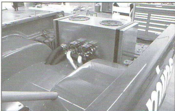
The intercooler water tank was mounted in the bed of the truck. An aerodynamic tonneau-type cover was fitted over the bed for the speed record runs.
