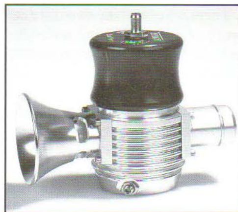
A dual-port unit features sequentially staged venting. During normal driving, excess pressure is returned to the intake tract via the BPV port shown here on the right side of the unit. During higher pressure events, the left-side BOV-type port is also opened, allowing additional venting. (Turbosmart)
