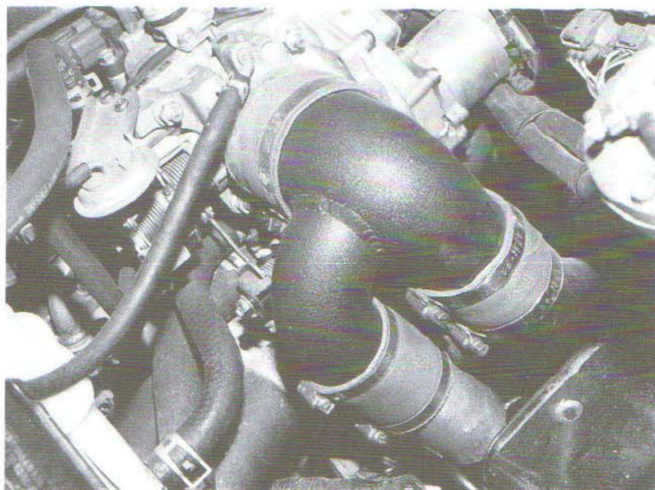
Fig. 17-15. Plumbing from the intercoolers unites in a single inlet to the throttle body. The mechanism attached to the forward side of the throttle inlet casting is an overboost safety vent valve.
