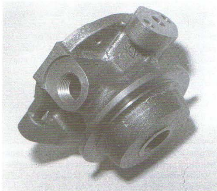
Fig. 3-15. The turbo bearing section with a water jacket offers extended turbo life and longer oil-change intervals.
