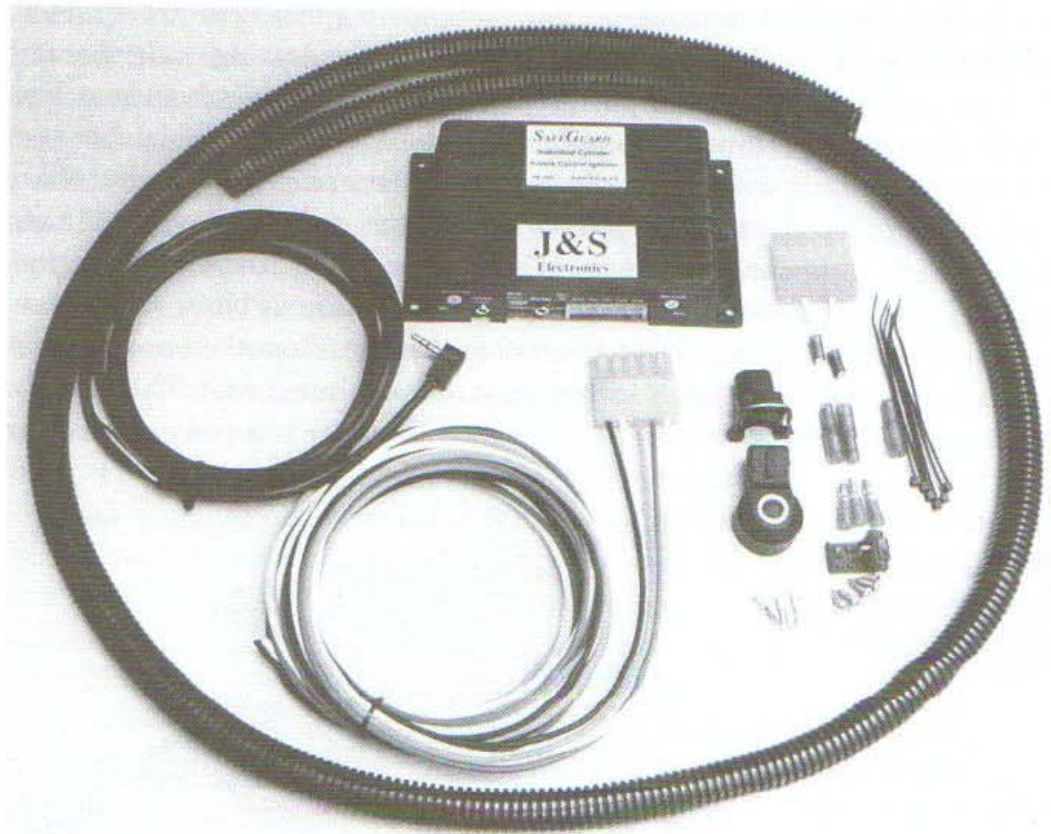
Fig. 9-4. An active knock-detection system with control of ignition timing is an excellent means of establishing a margin of safety for an engine. These items often add power as well as safety, by permitting ignition timing to stay closer to the knock threshold than is possible when tuning by ear.
