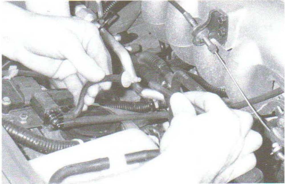
Fig. 18-26. The charcoal canister must be protected from boost pressure. A one-way valve placed in the vacuum line allows the engine to purge the canister while blocking boost pressure.
