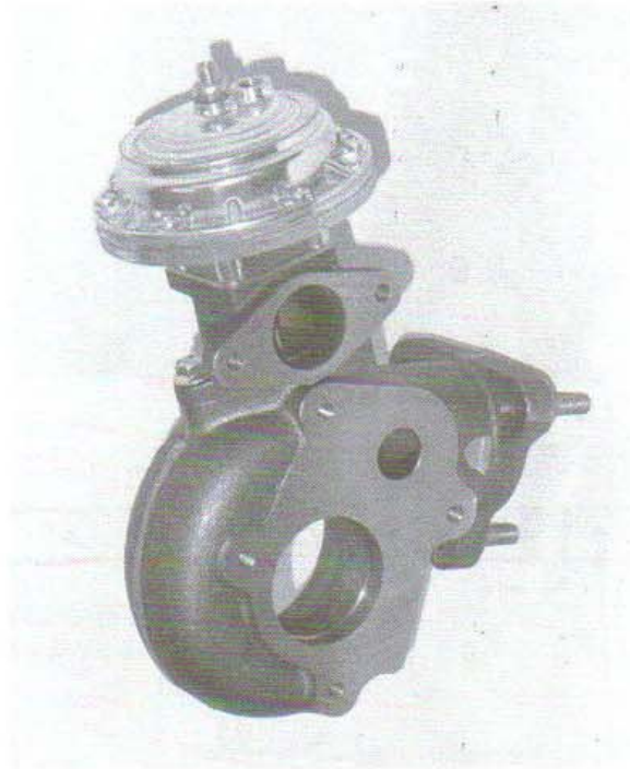
Fig. 12-13. A variation on the integral wastegate, but with a separate vent path
