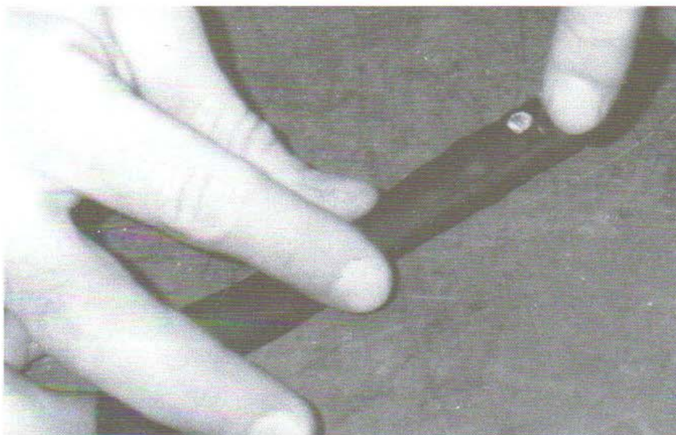
Fig. 18-21. The valve cover breather has a small restrictor inside that must be placed inside the new breather hose. The breather must be placed before the turbo to avoid pressurizing the crankcase.
