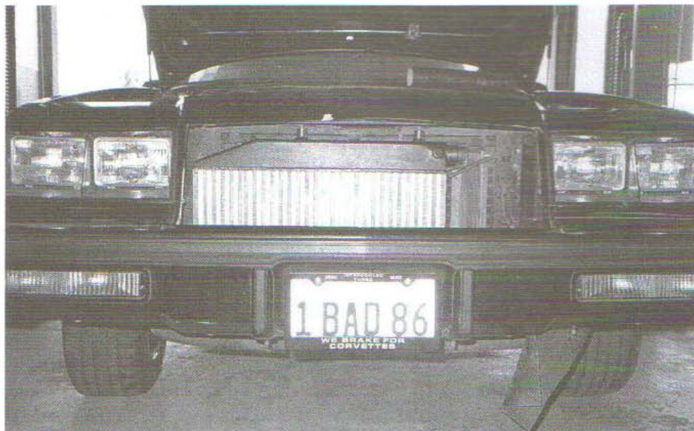
Fig. 5-2. The front-mounted intercooler is a typical aftermarket replacement for the Buick GN/GNX series cars.
