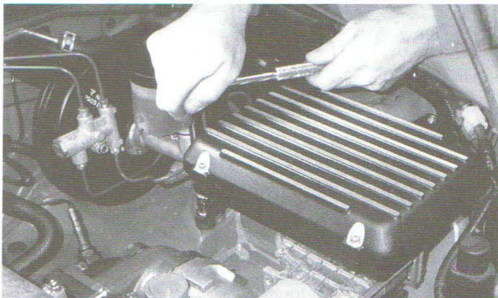
Fig. 18-20. The flow-meter/filter case assembly mounts to the Miata's structure with rubber isolators to allow for engine rock.
