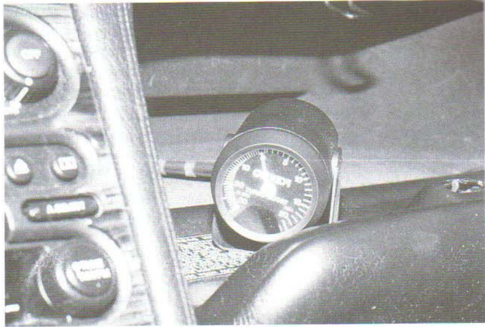
Fig. 17-21. The vacuum/boost gauge is not used frequently and is therefore mounted in the glove box, where it can be referred to if necessary.
