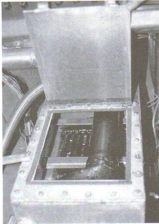
Fig. 5-38. An ice-chest heat exchanger for a one-shot intercooler for drag racing. Ice is packed around the water tubes, and the container is then filled with water.
