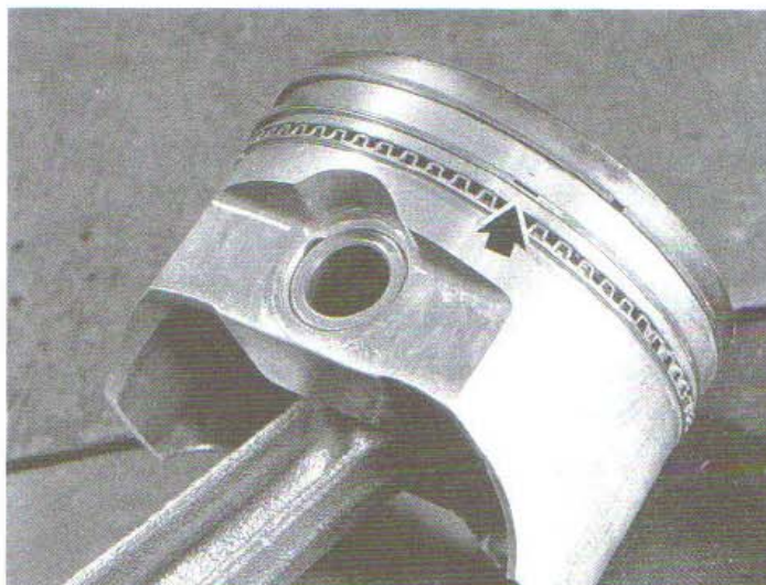
Fig. 13-10. A good turbo piston will have thick, strong ring lands.
