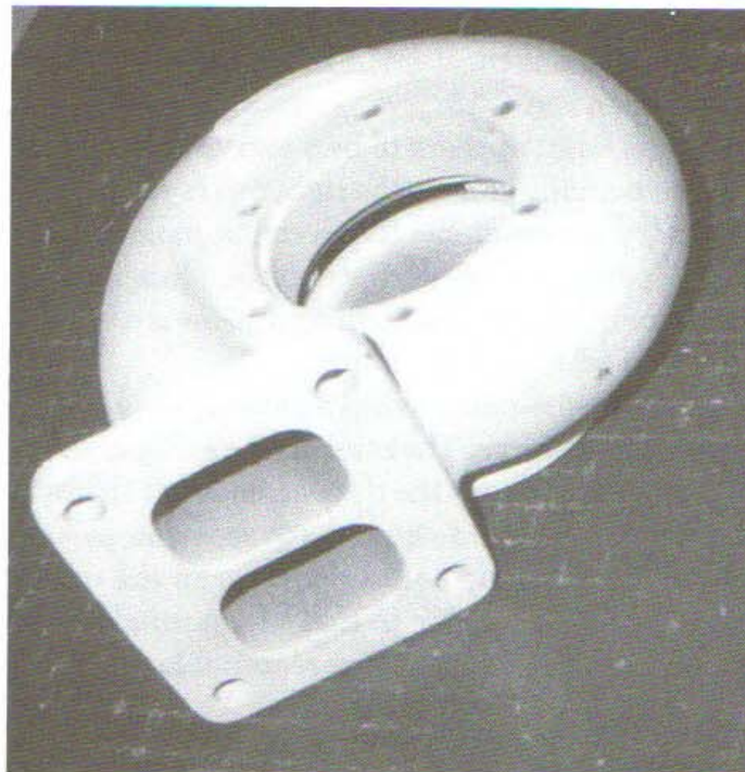
Fig. 3-14. The split-inlet exhaust housing theoretically offers a small performance advantage by keeping exhaust pulses in a tight bundle all the way to the turbine. This is more effective for engines with fewer cylinders, and thus fewer pulses, per engine cycle.
